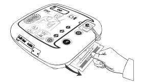
3. Insert the pad connector of the new pad into the Defibrillator Pads Connector, and then put the pad package in the Pads Storage Compartment as illustrated below.
